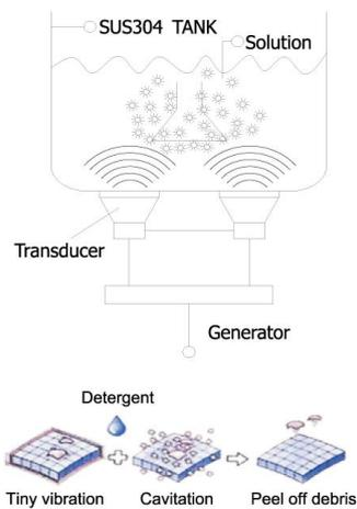
Ultrasonic cleaning is based on the cavitation effect caused by high frequency ultrasonic wave vibration signal in the fluid. Microscopic bubbles are formed, and then implode violently causing the cavitation which creates an intense scrubbing action on the surface of the item being cleaned. The bubbles are small enough to penetrate microscopic crevices, cleaning them thoroughly and consistently.
